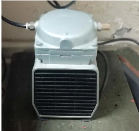
Air Assist Compressor
